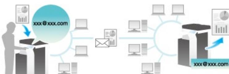
Within your intranet, the IP Address Fax function can be used. For IP Address Fax, specify either the IP address, host name or E-mail address of the destination fax machine to directly send a fax to that destination. No mail server is required.
