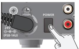
3. Turn on the power in the order of source devices → output devices.
