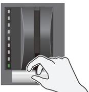
The video on the PGM/A bus is the final output. When the video fader is pushed all the way down, only the topmost or bottommost transition indicator lights.
