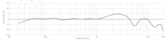
Note: Frequency response is measured with attached foam cap
