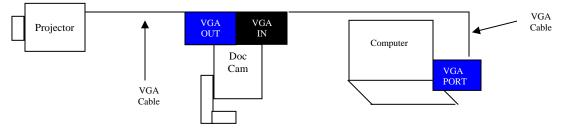
\* Active pass-through feature is unavailable when document camera is connected to a TV unless a PC to TV converter (AVerKey) is used.
