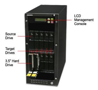
The **SOURCE** drive is the far left unit on the top array, the **TARGET** drives are the remaining four units on the top array and all five units on the bottom.
